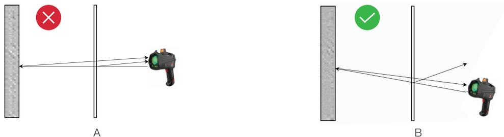
Figure 4.6 Do's and Don'ts when detecting through the glass
